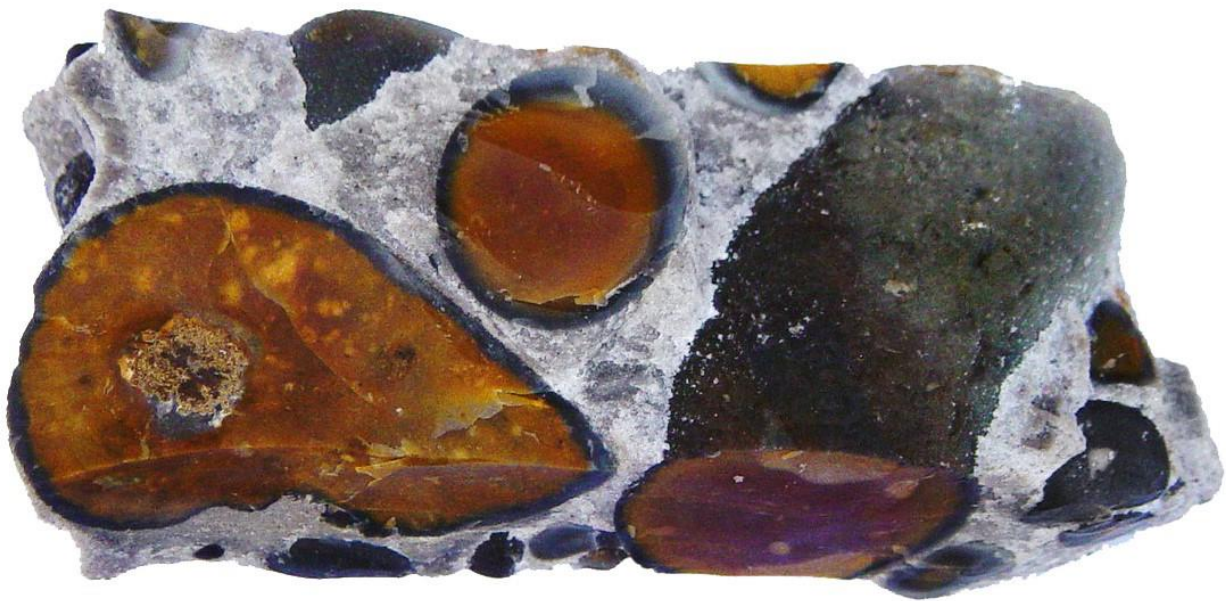
Hertfordshire Puddingstone from roof collapse
